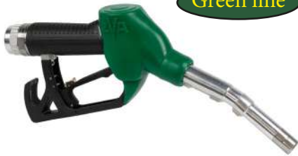
ZVA DN 16 auto nozzle Capacity: 60L/min Swivel: 1" or \frac{3}{4} " Spouts: 16 mm (unleaded)
